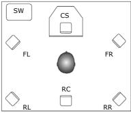
Figure 2-10: Recommended speaker placement.
